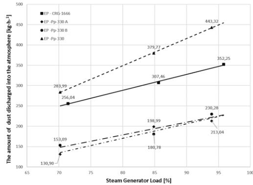
Fig. 11. The Amount of Dust Discharged
