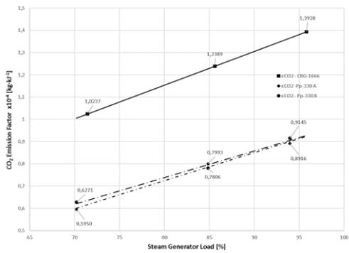
Fig. 4. CO<sub>2</sub> Emission Factor
