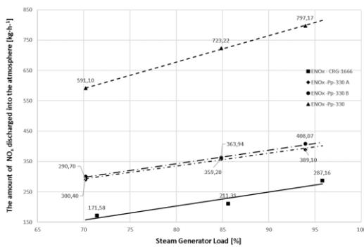
Fig. 10. The Amount of NO<sub>x</sub> Discharged
