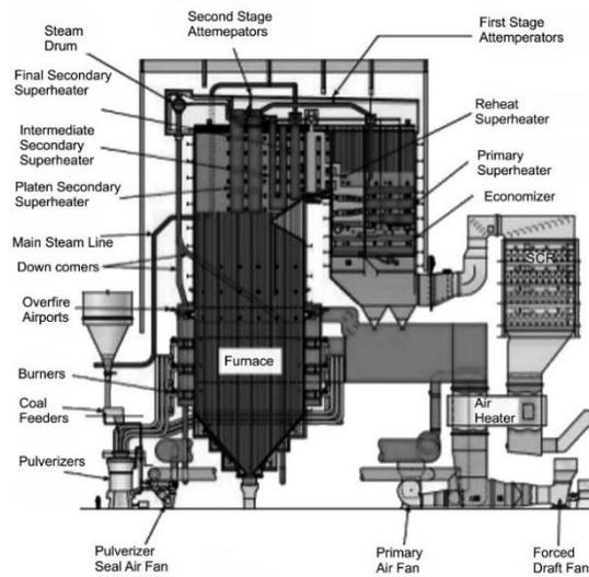
Fig. 2. Water tube boiler (steam generator) [3]
